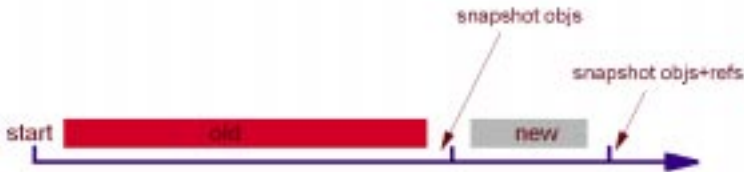
Fig. 3. Timeline of program execution: old objects are created before, and new objects during a critical operation
